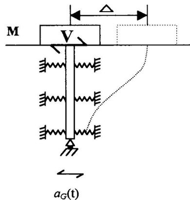
Figure 2: Pile in an Earthquake Excitation
